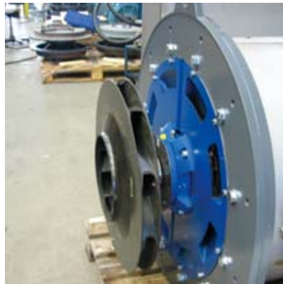
The impellers are manufactured from carbon fibre reinforced epoxy. There are two impellers in the ComVel-i unit, one for each stage.
